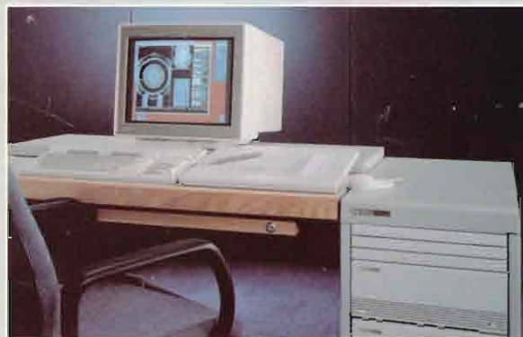
The HP 9000 Model 834CH is an HP-PA-based workstation that operates at 14 mips.
